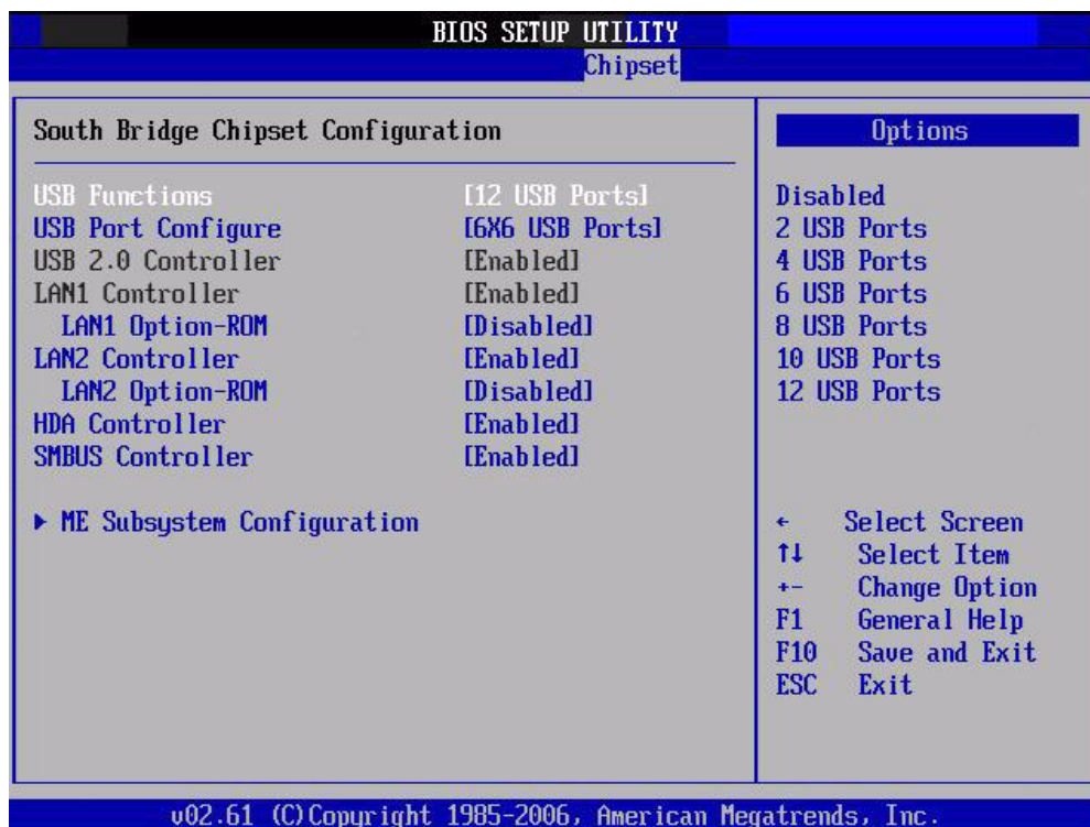
Figure 3.23 South Bridge Configuration
